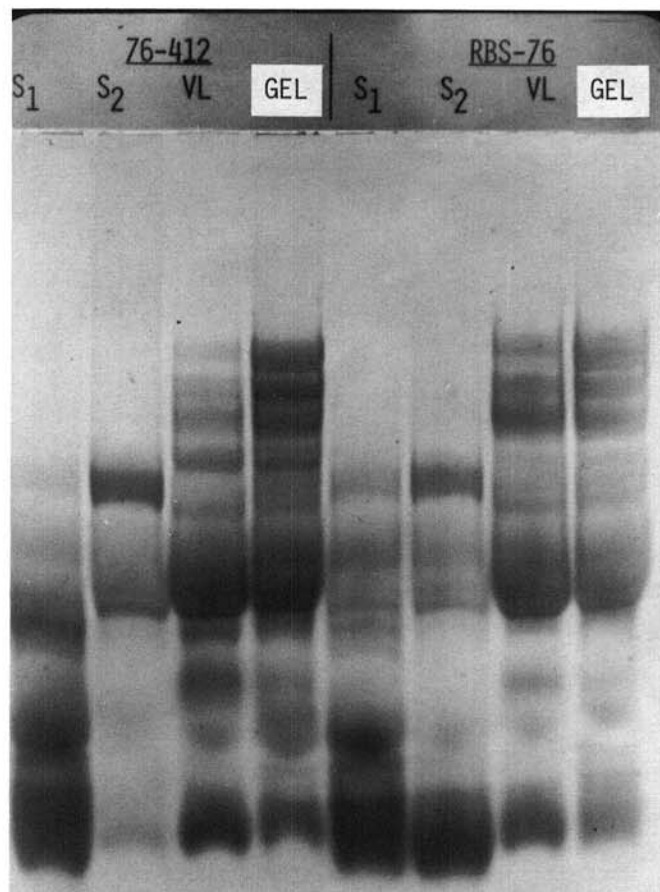
Fig. 6. Sodium dodecyl sulfate polyacrylamide gel electrophoresis patterns of proteins from various fractions, separated by ultracentrifugation, of acid-soluble gluten from RBS-76 (good baking quality) and 76-412 (poor baking quality) flours. Fractions were freeze-dried and collected as follows: S 1 , top three quarters of supernatant; S 2 , bottom quarter of supernatant; VL = viscous layer.
