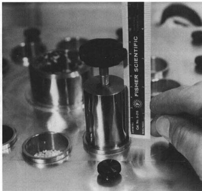
Fig. 8. Relative grain height measurement (50.8 mm) taken in a sample cup with the stainless steel plunger and ruler.
