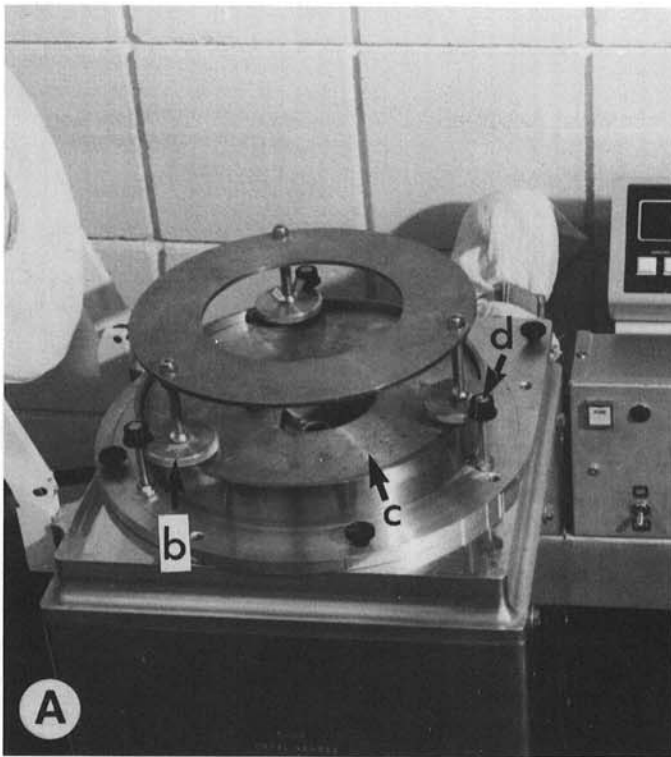
Fig. 5. Photograph illustrating the single-track plate mounted on the Tangential Abrasive Dehulling Device A , with and B , without the cover plate; a , grain in track; b , adjustable nut used for regulating the height of the ring, c , above the grain; d , retaining knob used to secure the adjustable nut; e , fan; and f , fan well.
