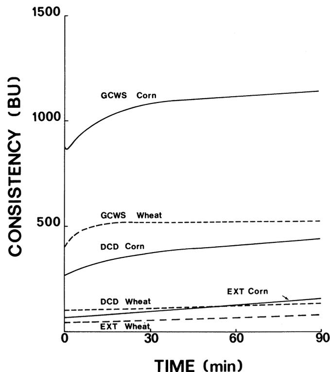
Fig. 2. Cold-paste (30°C) amylograms of "precooked" starches at 7.5% solids. GCWS = granular cold-water soluble; DCD = drum cooked and dried; EXT = extruded at 175°C and 18% moisture. BU = Brabender units.
