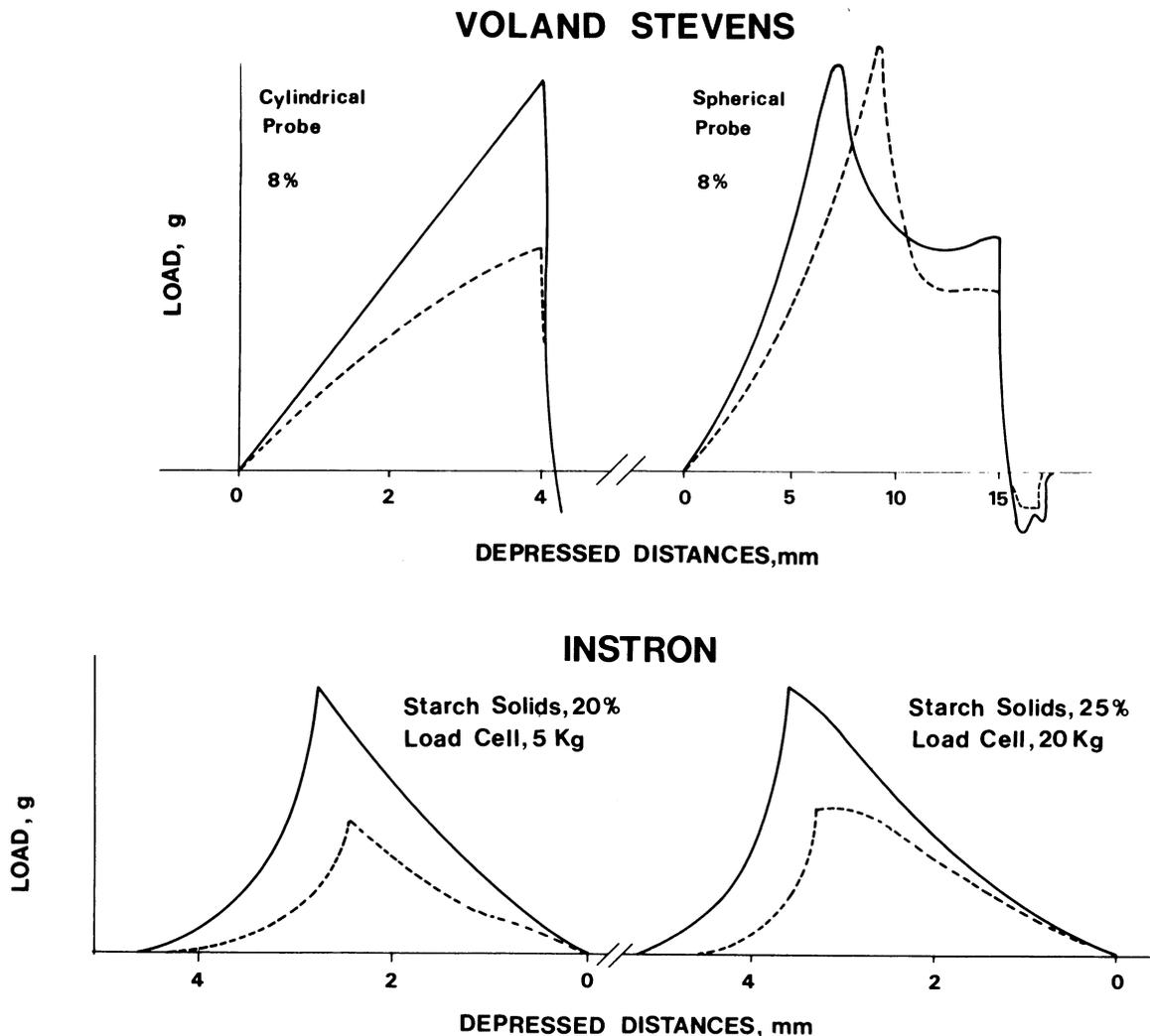
**Fig. 13.** Force-distance curves (Instron) for 20 and 25% gels made in 1% carboxymethylcellulose and aged 24 hr at 25°C. The yield stress of a gel was calculated from the peak on a curve, and firmness from the load at 2-mm depression. Curves are for corn (-----) and wheat (—). Voland-Stevens curves are shown at the top for gels containing 8% solids.
