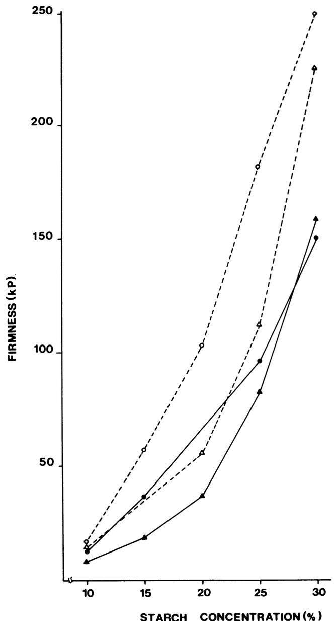
Fig. 12. Firmness (Instron) and yield force of gels made by cooking 10–30% starch in 1% aqueous carboxymethylcellulose and cooling 24 hr at 25°C ( $\Delta$ , yield force of corn;  $\circ$ , yield force of wheat;  $\blacktriangle$ , firmness of corn;  $\bullet$ , firmness of wheat).
