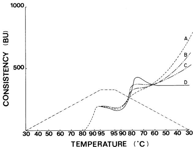
Fig. 8. Amylograms of wheat starch (7.5% solids) cooked to 95°C followed by addition of 0, 0.5, 1.0, and 2.0% wheat starch lipids (curves A, B, C, and D respectively), followed by cooling. BU = Brabender units.
