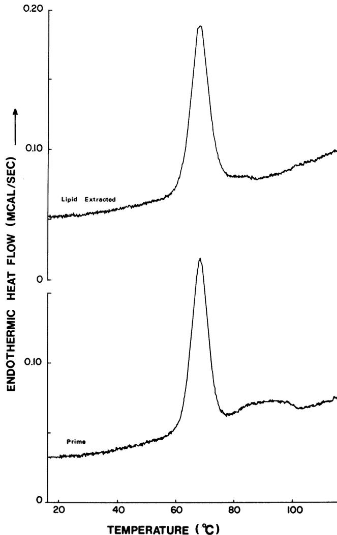
**Fig. 4.** Differential scanning calorimetry of prime corn starch and low-lipid corn starch at a water/starch ratio of 3:1 (w/w).
