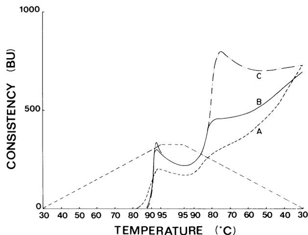
Fig. 7. Amylograms of wheat starch that had been previously impregnated with 0.5, 1.0, and 2.0% additional wheat starch lipids (curves A, B, and C, respectively). The total lipid contents, including the 1% native lipids, were approximately 1.5, 2.0, and 3.0%. All curves were run at 7.5% dry solids. BU = Brabender units.
