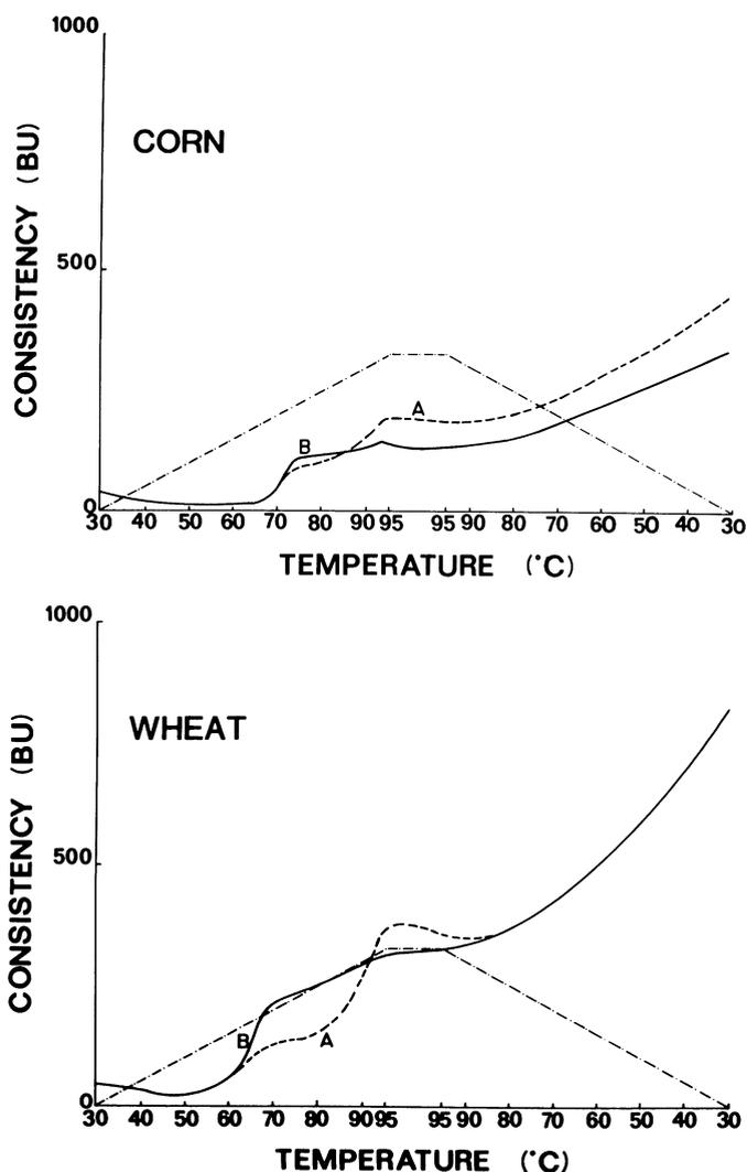
Fig. 5. Amylograms of corn and wheat starch (A) and low-lipid corn and low-lipid wheat starch (B) in 1% carboxymethylcellulose. BU = Brabender units.
