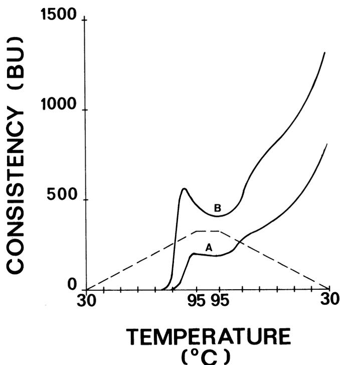
Fig. 1. Amylograms of wheat (A) and corn starch (B) at 7.5% solids in water. The dashed line is the temperature profile. BU = Brabender units.
