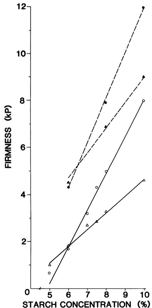
Fig. 10. Firmness (Voland-Stevens) of starch gels made with and without 1% carboxymethylcellulose, ( $\Delta$  and  $\circ$ , corn and wheat starch, respectively, in water;  $\blacktriangle$  and  $\bullet$ , corn and wheat starch, respectively, in 1% carboxymethylcellulose). kP = kilopoise.
