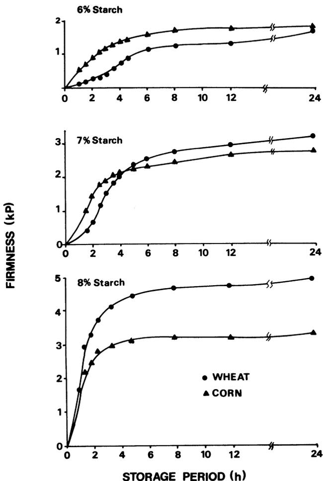
Fig. 11. Firmness (Voland-Stevens) of corn and wheat starch gels after aging 0–24 hr at 25°C. kP = kilopoise.
