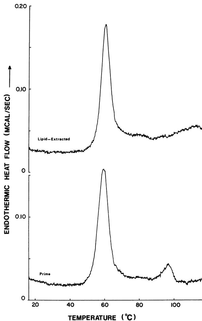
**Fig. 3.** Differential scanning calorimetry of prime wheat starch and low-lipid wheat starch at a water/starch ratio of 3:1 (w/w).
