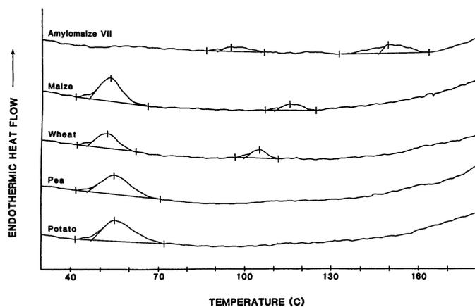
Fig. 1. Differential scanning calorimetry thermograms of autoclaved-cooled and freeze-dried starches from amylo maize VII, regular maize, wheat, pea, and potato.
