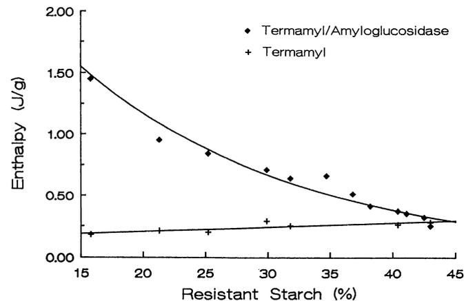
Fig. 5. Effects of enzyme-resistant starch content and different amylase applications on enthalpies of the transition at 54°C in enzyme-resistant starch residues from amylo maize VII starch preparations. Heating at a rate of 5°C/min in the differential scanning calorimeter with addition of water (starch/water ratio 1:3).
