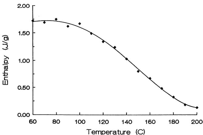
Fig. 4. Thermoreversibility of the endothermic transition at 54°C in vacuum-dried enzyme-resistant starch residue from native amylo maize VII starch. Heating at a rate of 5°C/min in the differential scanning calorimeter without addition of water.
