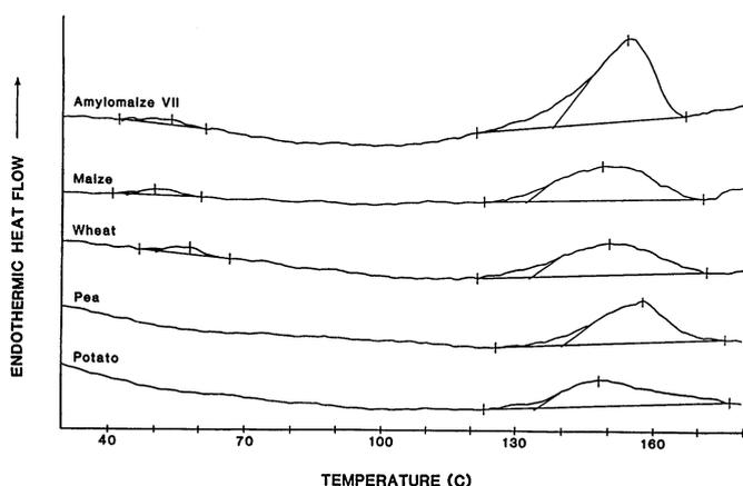
Fig. 2. Differential scanning calorimetry thermograms of enzyme-resistant starch residues isolated from autoclaved-cooled and freeze-dried starches from amylo maize VII, regular maize, wheat, pea, and potato.
