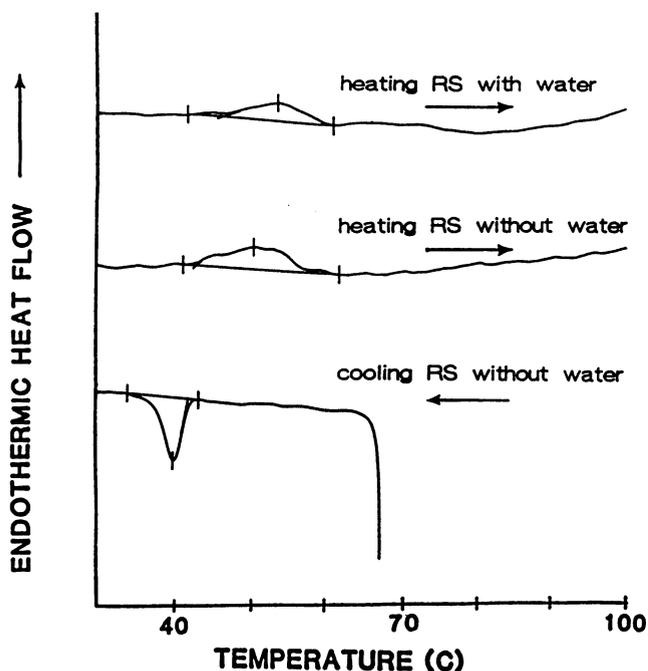
Fig. 3. Differential scanning calorimetry thermograms of enzyme-resistant starch residues isolated from native amylo maize VII starch. Heating and cooling rate: 5°C/min.
