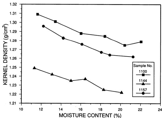
Fig. 3. Change in kernel density with moisture content for three of the 10 maize samples.
