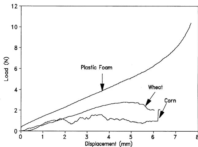
Fig. 3. Simple compression test curves of plastic foam and corn and wheat starch extrudates.
