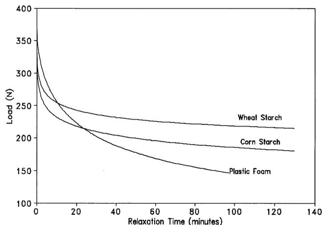
Fig. 4. Stress relaxation test curves of plastic foam and corn and wheat starch extrudates.
