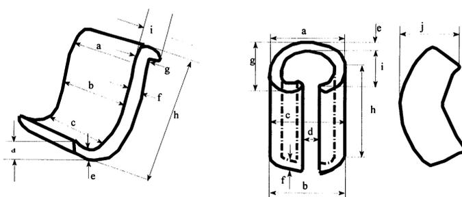
Fig. 1. Measurements made with a digital reading caliper of the dimensions of three types of cushioning materials. Measurements for each dimension were made at three different places and then averaged.
