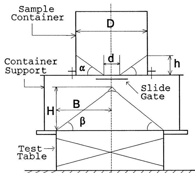
Fig. 1. Prototype for measuring repose angle ( $\beta$ ) and drain angle ( $\alpha$ ).
