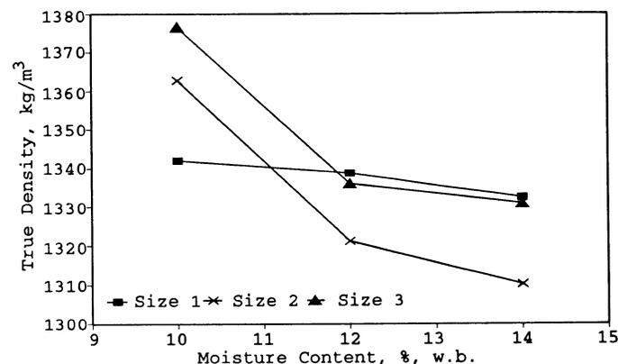
Fig. 3. True density of soybean meals at different moisture contents. Size 1: regular mixture of soybean meals; Size 2: soybean meal particles retained on U.S. no. 16 sieve; Size 3: soybean meal particles passed through U.S. no. 16 sieve.
