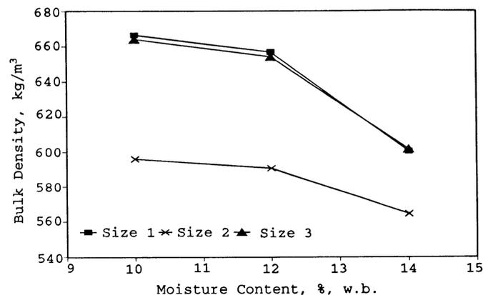
Fig. 4. Bulk density of soybean meals at different moisture contents. Size 1: regular mixture of soybean meals; Size 2: soybean meal particles retained on U.S. no. 16 sieve; Size 3: soybean meal particles passed through U.S. no. 16 sieve.
