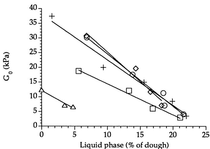
Fig. 6. Stress-relaxation modulus ( $G_0$ ) as a function of amount of separated liquid phase. Symbols as in Fig. 3.
