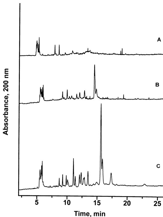
**Fig 6.** Capillary electrophoresis separation of rice cultivar IR-28 prolamins in three buffer systems: 100 mM phosphate buffer, pH 2.5, containing 0.05% hydroxypropylmethylcellulose (A); buffer A containing 20% acetonitrile (P-ACN) (B); and P-ACN + 26 mM lauryl-sulfobetain (C). Separations were carried out in 27-cm (20-cm separation length)  $\times$  50- $\mu$ m i.d. capillaries at 10 kV (+ to -) and 40°C. Samples were pressure-injected for 5 sec each.
