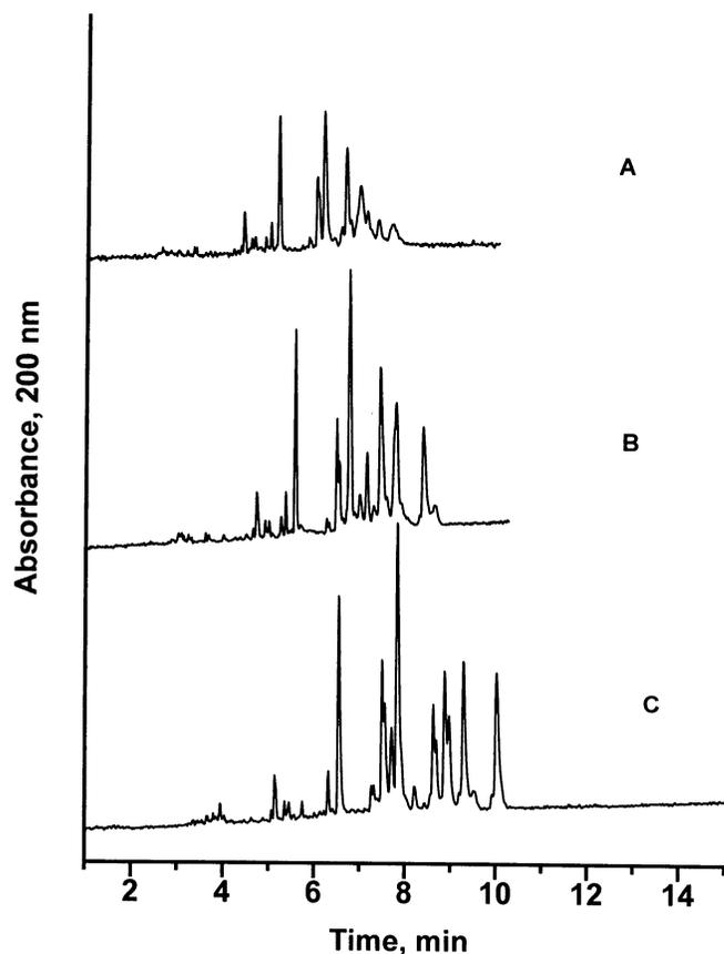
**Fig 5.** Capillary electrophoresis separation of oat cultivar Troy prolamins in three buffer systems: 100 mM phosphate buffer, pH 2.5, containing 0.05% hydroxypropylmethylcellulose (A); buffer A containing 20% acetonitrile (P-ACN) (B); and P-ACN + 26 mM lauryl-sulfobetain (C). Separation conditions same as for Fig. 1.
