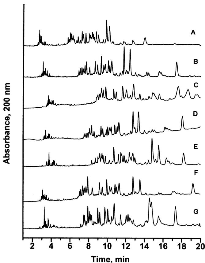
**Fig 3.** Capillary electrophoresis separations of TAM 107 gliadins using the following separation buffers: 100 mM phosphate buffer, pH 2.5, containing 0.05% hydroxypropylmethylcellulose (A); buffer A containing 20% acetonitrile (P-ACN) (B); P-ACN + 26 mM Brij-35 (C); P-ACN + 26 mM CHAPS (D); P-ACN + 26 mM hexane sulfonic acid (E); P-ACN + 26 mM octyl-sulfobetain (F); and P-ACN + 26 mM lauryl-sulfobetain (G). Separation conditions as in Fig. 1.
