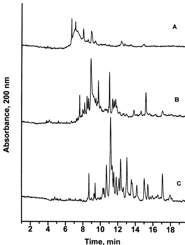
**Fig 4.** Capillary electrophoresis separations of TAM 107 glutenins in three buffers systems: 100 mM phosphate buffer, pH 2.5, containing 0.05% hydroxypropylmethylcellulose (A); buffer A containing 20% acetonitrile (P-ACN) (B); and P-ACN + 26 mM lauryl-sulfobetain (C). Separation conditions as in Fig. 1.
