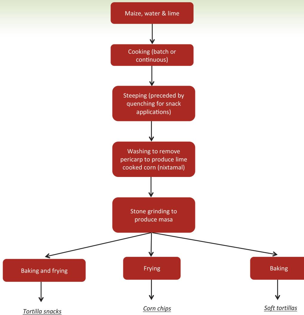
Fig. 4. Steps in alkaline lime-cooking of maize (nixtamalization process).
