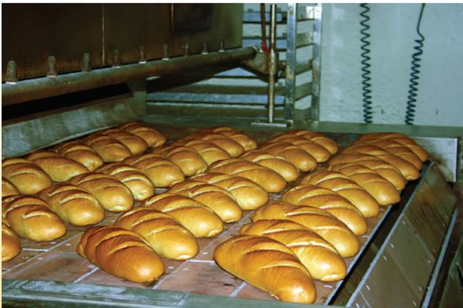
Fig. 1. Baked product exiting a tunnel oven.
