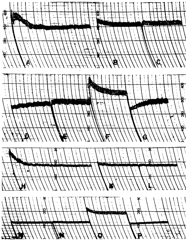
Fig. 1. Farinograms of starch-water mixtures. Series A to G: 300 g. wheat starch (14% m.b.) plus 176 g. water; series H to P: plus 1% GMS. Mixing time, 10 minutes for A and H, 5 minutes for the other curves; mixing speed, 58 r.p.m. for A, B, C, F, H, K, L, and O; 29 r.p.m. for D, E, G, M, N, and P; in the case of B, D, K, and M, mixing was preceded by 5 minutes' dough rest; after the recording of curves B, D, H, and M, mixing was interrupted for 20 seconds; for the rest, mixing proceeded without interruption.
