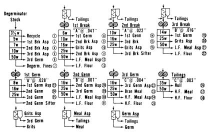
Fig. 1. Roller-milling and grading flowsheet. Degermer stock from yellow and white corn infected with *H. maydis* was milled into grits, meal, and other products in this manner. Brk = break; Asp = aspirator; L. F. Meal = low-fat meal; H. F. Meal = high-fat meal; w = wire mesh, e.g. number of wire meshes per lineal inch of sieve surface.
