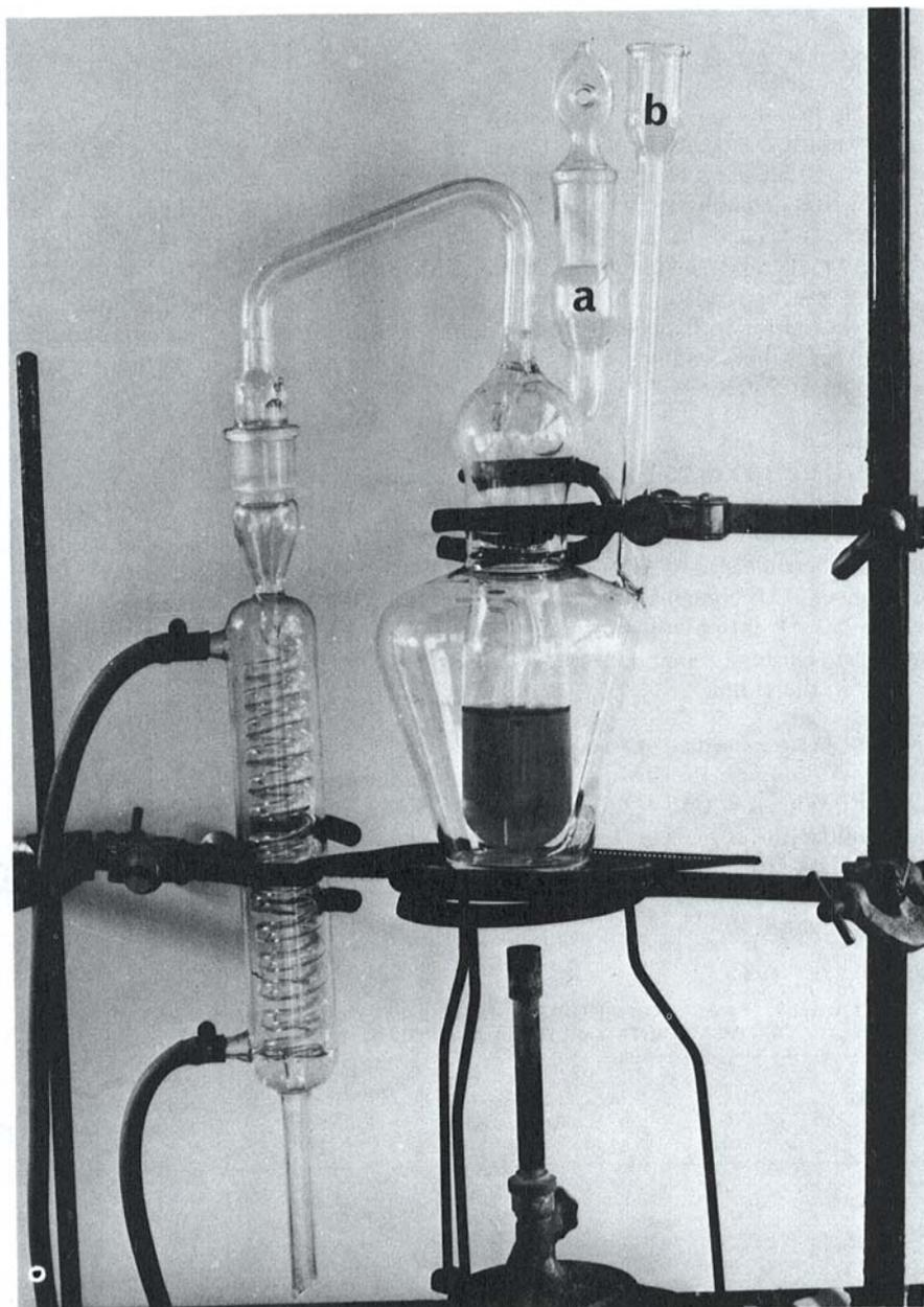
Fig. 1. Apparatus for steam distillation according to Duffau (6).
