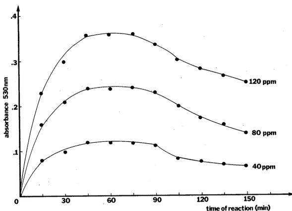
Fig. 2. Reaction of furfural and the aniline acetate reagent at 25°C. as a function of time.
