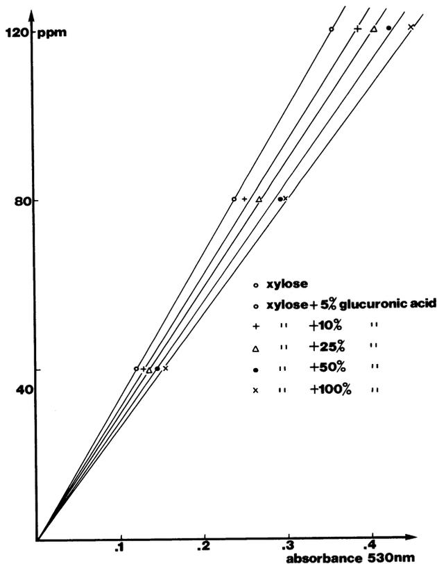
Fig. 3. Influence of glucuronic acid on the color reaction with the aniline acetate reagent.
