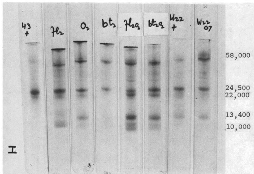
Fig. 2. Acrylamide gel patterns of protein polypeptides derived from Fraction I of corn endosperms.
