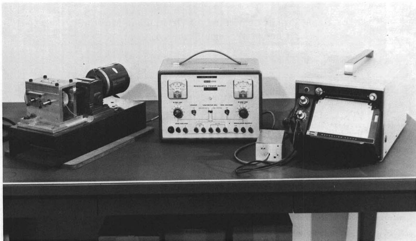
Fig. 1. Instrument for determining moisture content of single kernels of corn with rolls (left), power supply (center), and high-speed recorder (right).
