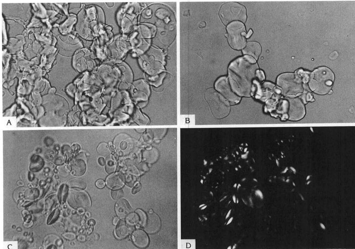
Fig. 1. Wheat starch, water, oil samples heated to 68°C in a differential scanning calorimeter and redispersed in oil for microscopy. A, Control, no oil present during heating; B, coconut oil; C, soybean oil; D, soybean oil, polarized light.
