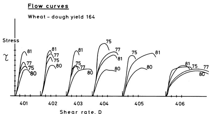
Fig. 3. Flow curves from meal doughs with constant water absorption (six wheat varieties or selections for four years).
