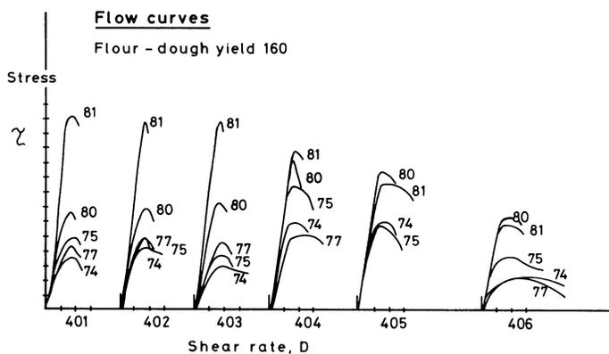
Fig. 4. Flow curves from flour doughs with constant water absorption (six wheat varieties for five years).
