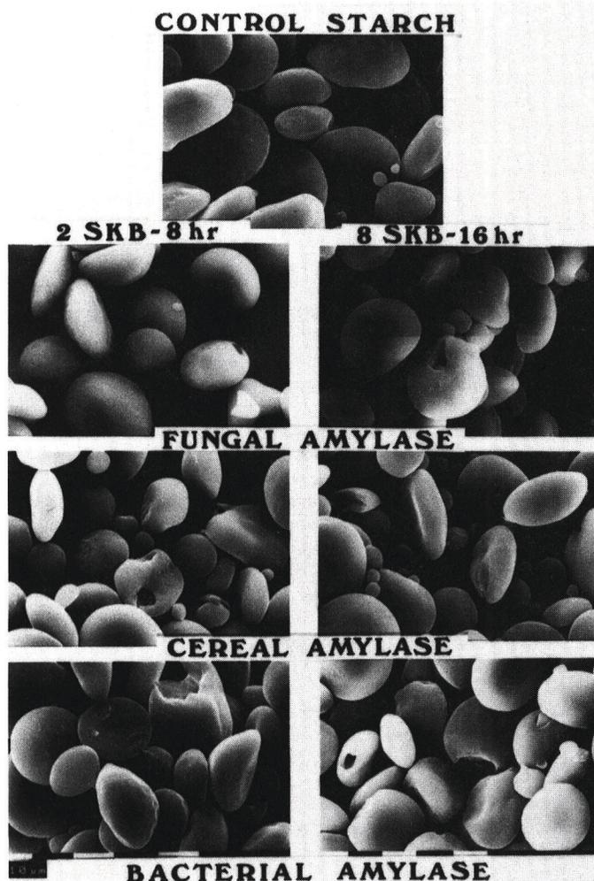
Fig. 2. Scanning electron micrographs of control and selected enzyme treated starches.
