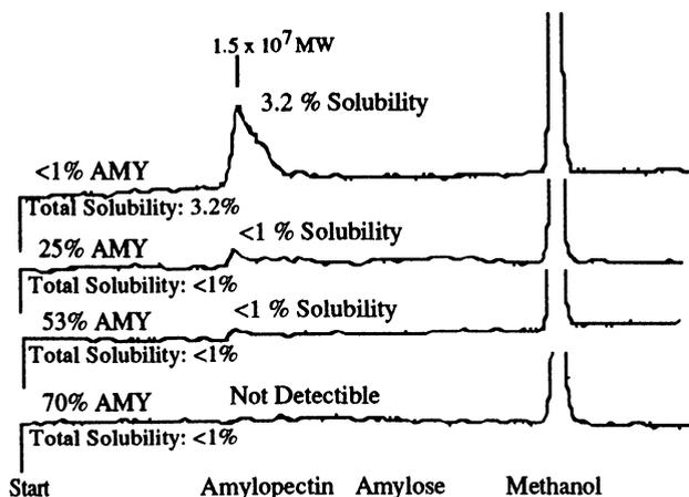
Fig. 3. High-performance size-exclusion chromatography solubility profiles of corn starch (1%) extracted at 65°C for 10 min and sonicated 20 sec. Data include total starch solubility, solubility of amylose (AMY) and amylopectin (AMP), and apparent molecular weights (MW).
