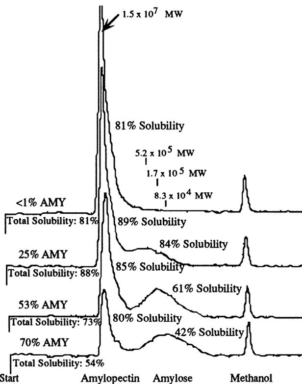
Fig. 5. High-performance size-exclusion chromatography solubility profiles of corn starch (1%) boiled for 10 min, autoclaved for 10 min, and sonicated 20 sec. Data include total starch solubility, solubility of amylose (AMY) and amylopectin (AMP), and apparent molecular weights (MW).
