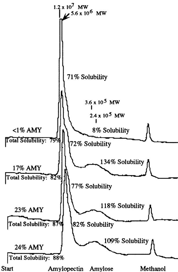
Fig. 7. High-performance size-exclusion chromatography solubility profiles of sorghum starch (1%) boiled for 10 min, autoclaved for 10 min, and sonicated 20 sec. Data include total starch solubility, solubility of amylose (AMY) and amylopectin (AMP), and apparent molecular weights (MW). AMY solubility includes low-MW AMP. The amount of soluble low-MW AMP from waxy starch (<1% AMY) is presented.
