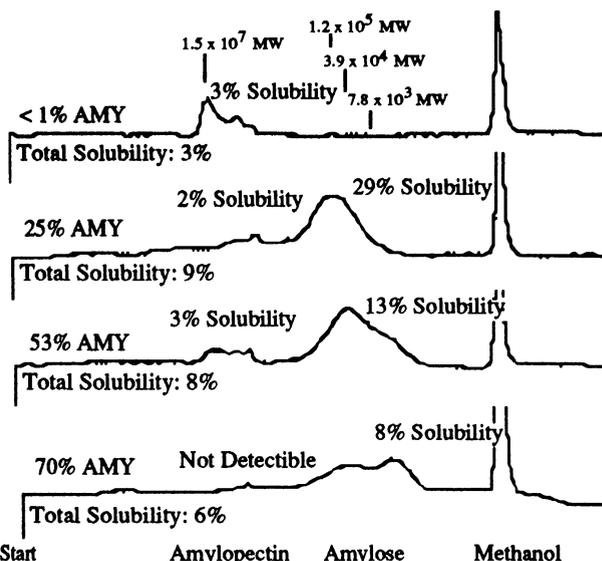
Fig. 2. High-performance size-exclusion chromatography solubility profiles of corn starch (1% solutions) extracted at 85°C by aqueous leaching for 4 hr. Data include total starch solubility, solubility of amylose (AMY) and amylopectin (AMP), and apparent molecular weights (MW).
