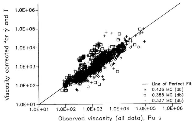
**Fig. 2.** Viscosity corrected for shear rate and temperature versus all data.
