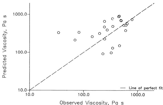
Fig. 6. Predicted versus observed viscosities corrected for shear rate, temperature, moisture, and time-temperature history in extruder dies for whole wheat flour doughs.
