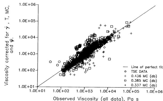
Fig. 5. Viscosity corrected for shear rate, temperature, moisture content, and time-temperature history for all data.
