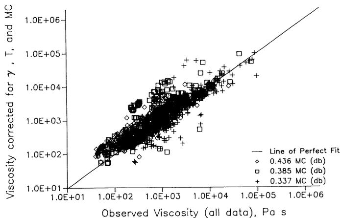
**Fig. 3.** Viscosity corrected for shear rate, temperature, and moisture content versus all data.
