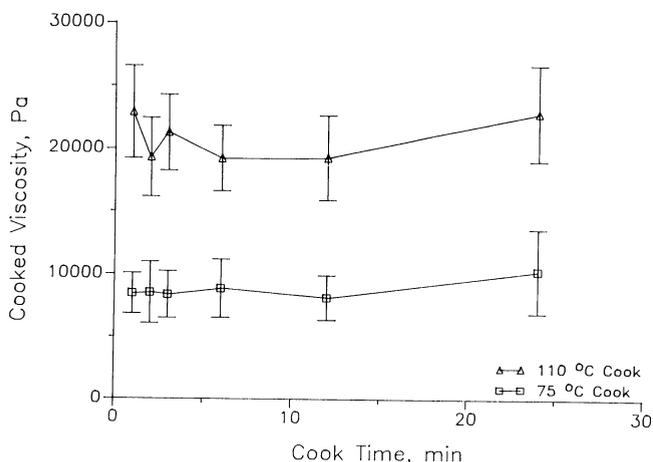
Fig. 4. Cooked whole wheat flour viscosity versus cook time at 100 sec<sup>-1</sup> and 0.443 g of water per gram of flour moisture content.
