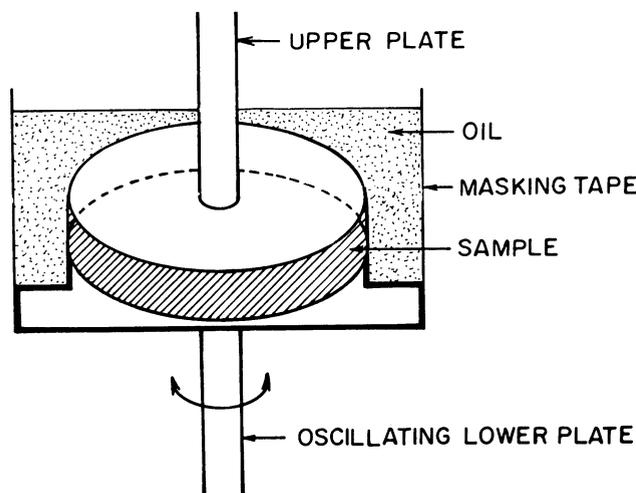
Fig. 1. Fixture geometry configuration of the measuring system indicating the positioning of the sample and the covering thin layer of mineral oil.
