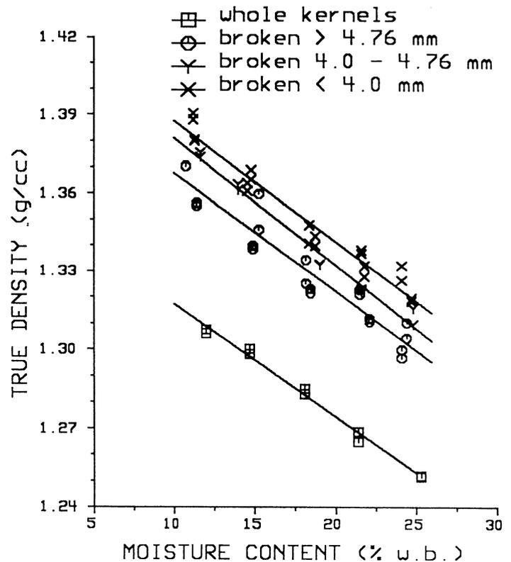
Fig. 5. Relationship between true density and moisture content for various fractions of corn.
