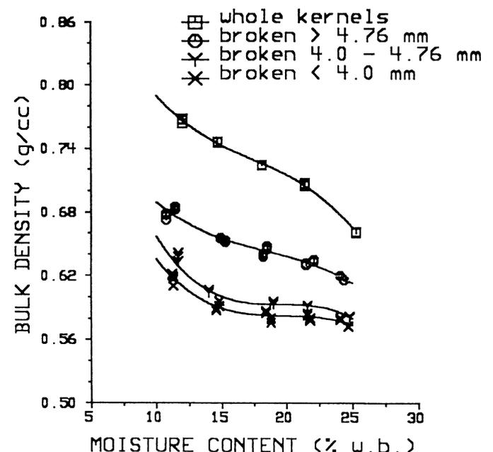
Fig. 6. Relationship between bulk density and moisture content for various fractions of corn.
