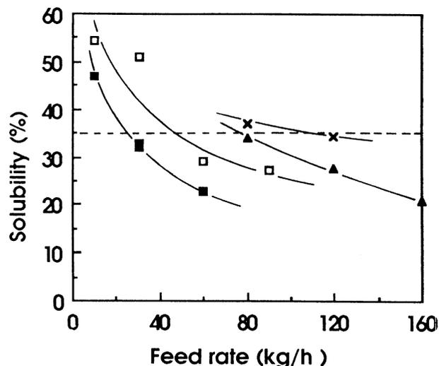
Fig. 3. Compared evolutions of extrudate solubility on BC 45 and BC 72: BC 45, one reverse screw element (RSE), 8 mm-wide slots, 200 rpm (■); BC 45, 2 RSE, 8-mm-wide slots, 200 rpm (□); BC 72, 1 RSE, 14-mm-wide slots, 130 rpm (▲); BC 72, 2 RSE, 8-mm-wide slots, 130 rpm (x).
