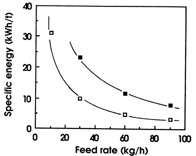
Fig. 10. Influence of number of reverse screw elements (RSE) on computed specific mechanical energy. BC 45, 8-mm-wide slots, rotation speed = 200 rpm: 1 RSE (□), 2 RSE (■).
