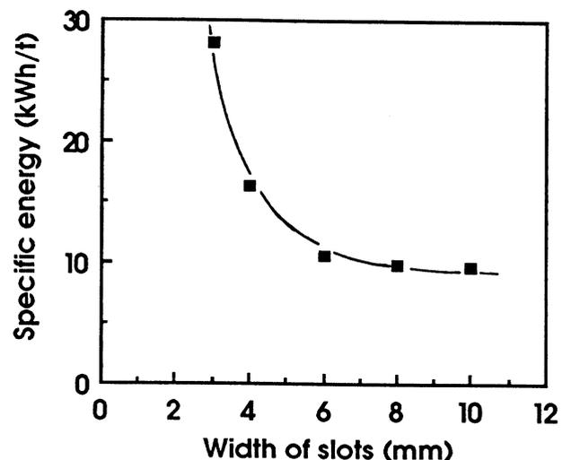
Fig. 11. Influence of slot width on computed specific mechanical energy. BC 45, one reverse screw element, feed rate = 30 kg/hr, rotation speed = 200 rpm.
