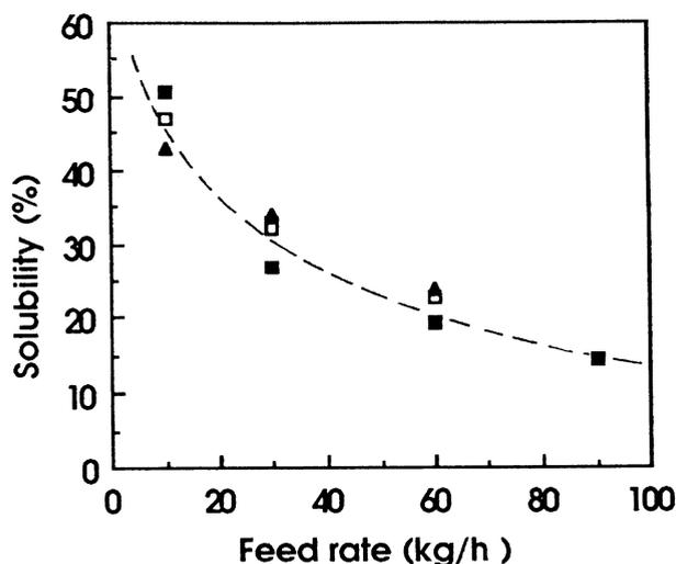
Fig. 1. Influence of feed rate and rotation speed on extrudate solubility. BC 45, one reverse screw element, 8-mm-wide slots: 250 rpm (■), 200 rpm (□), 150 rpm (▲).
