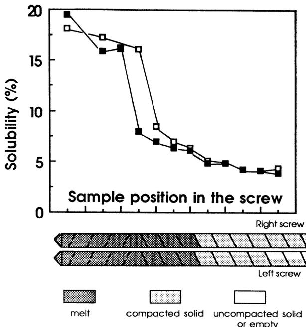
Fig. 4. Evolution of solubility along the screw. BC 45, 1 RSE, 10-mm-wide slots, feed rate = 30 kg/hr, rotation speed = 100 rpm: right screw (□), left screw (■).
