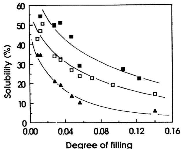
Fig. 2. Influence of degree of filling and number of reverse screw elements (RSE) on extrudate solubility. BC 45, 8-mm-wide slots: 2 RSE (■), 1 RSE (□), 0 RSE (▲).
