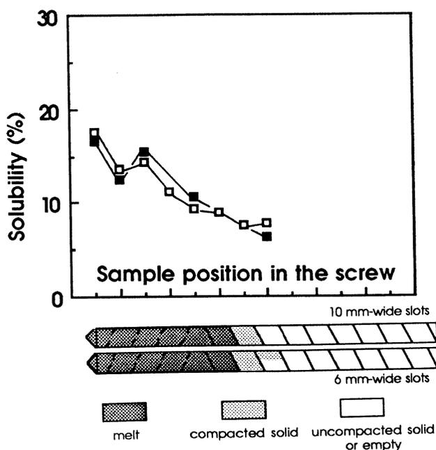
Fig. 7. Influence of slot widths on solubility and degree of filling. BC 45, one reverse screw element, feed rate = 30 kg/hr, rotation speed = 200 rpm: 6 mm (■), 10 mm (□).
