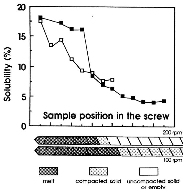
Fig. 5. Influence of rotation speed on solubility and degree of filling. BC 45, one reverse screw element, 10-mm-wide slots, feed rate = 30 kg/hr: 200 rpm (□), 100-rpm (■).
