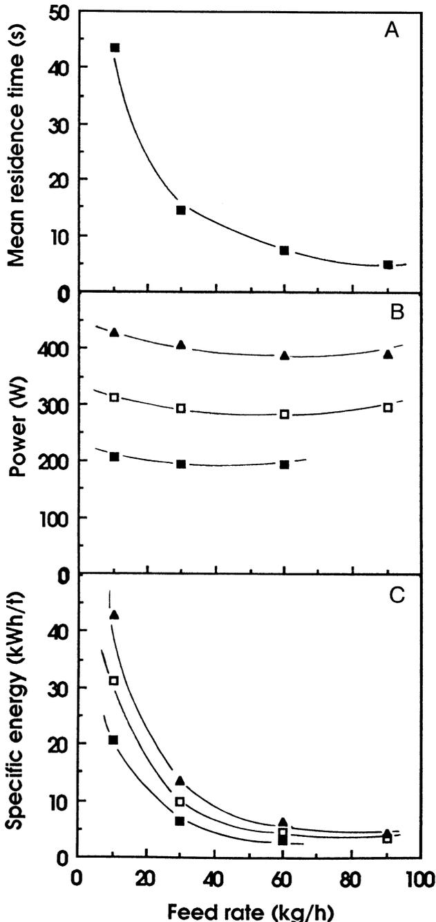
Fig. 9. Influence of feed rate and rotation speed on A, computed mean residence time; B, dissipated power; and C, specific mechanical energy. BC 45, one reverse screw element, 8-mm-wide slots: 150 rpm (■), 200 rpm (□), 250 rpm (▲).
