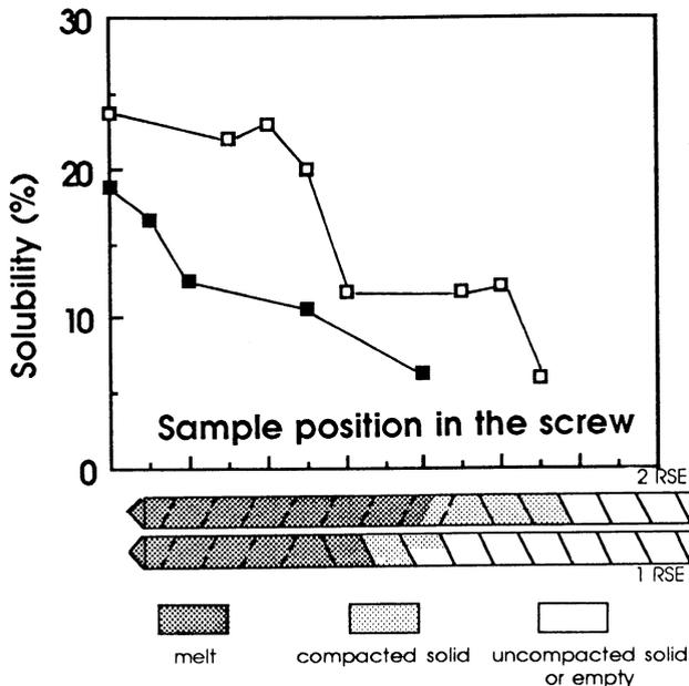
Fig. 6. Influence of reverse screw element (RSE) length on solubility and degree of filling. BC 45, 6-mm-wide slots, feed rate = 30 kg/hr, rotation speed = 200 rpm: 1 RSE (■), 2 RSE (□).
