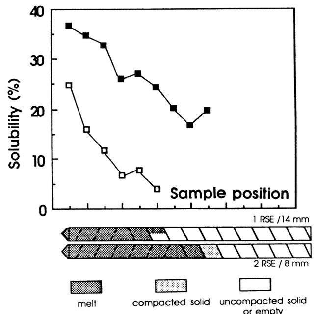
Fig. 8. Influence of reverse screw element (RSE) configuration on solubility and degree of filling. BC 72, feed rate = 80 kg/hr, rotation speed = 130 rpm. Moisture content = 17.6% (wb): 1 RSE, 14-mm-wide slots (□); 2 RSE, 8-mm-wide slots (■).
