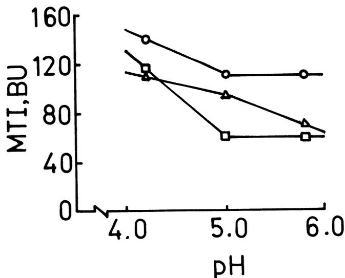
Fig. 3. Effect of pH and salt on the mixing tolerance index (MTI) values (BU) of high  $\alpha$ -amylase flour containing 540 SKB units per 100 g. Salt: 0.0 (○—○), 1.5 (△—△), 2.5 (□—□).
