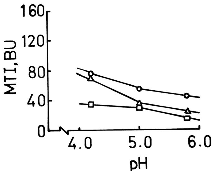
Fig. 1. Effect of pH and salt on the mixing tolerance index (MTI) values (BU) of control flour. Salt: 0.0 (○—○), 1.5 (△—△), 2.5 (□—□).
