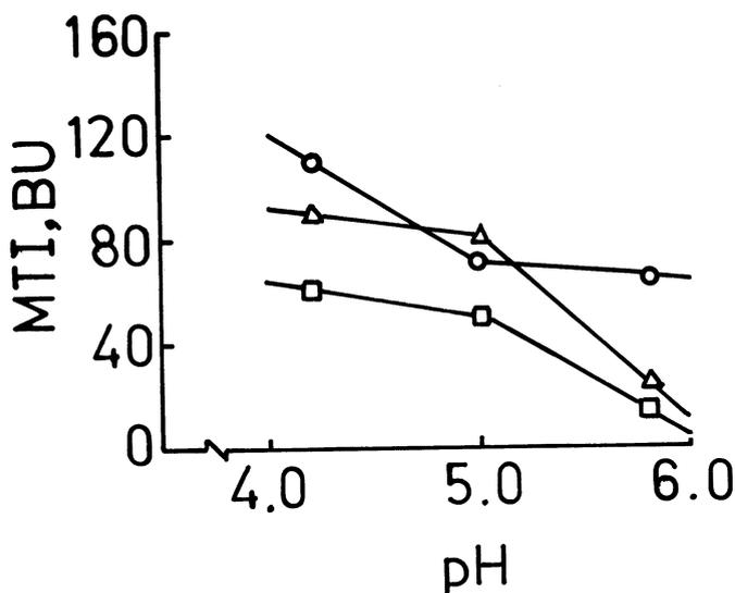
Fig. 2. Effect of pH and salt on the mixing tolerance index (MTI) values (BU) of high  $\alpha$ -amylase flour containing 108 SKB units per 100 g. Salt: 0.0 (○—○), 1.5 (△—△), 2.5 (□—□).
