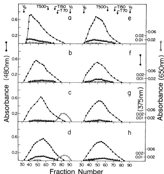
Fig. 3. Chromatography on a Sepharose CL-4B column ( $2.5 \times 85$  cm, eluted with 0.3% NaCl and 0.05%  $\text{NaN}_3$ , flow rate 25 ml/hr,  $25^\circ\text{C}$ ) of arabinoxylans isolated from various flours. a, Katepwa; b, Glenlea; c, Marshall; d, Fielder; e, HY 355; f, HY 320; g, Oslo; h, Norstar. Absorbance at 480, 375, and 650 nm corresponds to eluting carbohydrates (●), ferulic acid (▲), and proteins (○), respectively.
