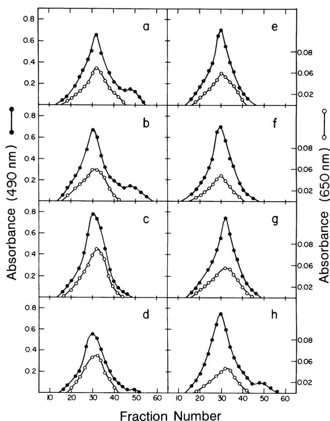
**Fig. 4.** Chromatography on a Sephacryl S-300 column (2.5 × 85 cm, eluted with 0.3% NaCl and 0.05% NaN<sub>3</sub>, flow rate 25 ml/hr, 25°C) of arabinogalactans isolated from various flours. a, Katepwa; b, Glenlea; c, Marshall; d, Fielder; e, HY 355; f, HY 320; g, Oslo; h, Norstar. Absorbance at 490 and 650 nm corresponds to eluting carbohydrates (●) and proteins (○), respectively.
