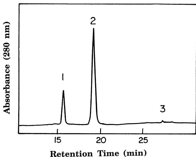
Fig. 1. High-performance liquid chromatogram of deesterified phenolic acids from arabinoxylan (Katepwa). 1, *cis*-ferulic acid; 2, *trans*-ferulic acid; 3, *trans*-cinnamic acid.
