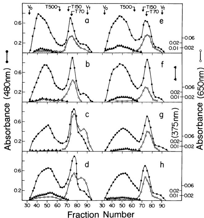
Fig. 2. Chromatography on a Sepharose CL-4B column ( $2.5 \times 85$  cm, eluted with 0.3% NaCl and 0.05%  $\text{NaN}_3$ , flow rate 25 ml/hr,  $25^\circ\text{C}$ ) of pentosans isolated from various flours. a, Katepwa; b, Glenlea; c, Marshall; d, Fielder; e, HY 355; f, HY 320; g, Oslo; h, Norstar. Absorbance at 480, 375, and 650 nm corresponds to eluting carbohydrates (●), ferulic acid (▲), and proteins (○), respectively.
