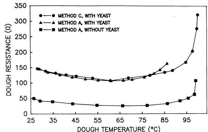
Fig. 7. Electrical resistances in doughs containing yeast during baking with methods A and C compared with those of unyeasted doughs during baking with method A.
