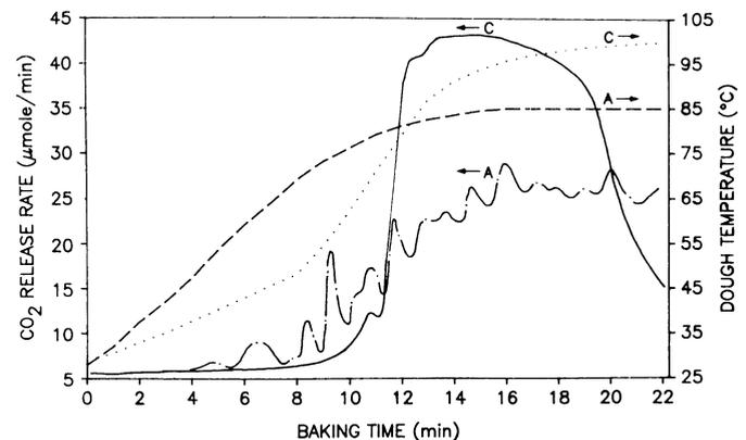
Fig. 6. Effect of heating method on CO<sub>2</sub> loss from dough during baking in an electric resistance oven.
