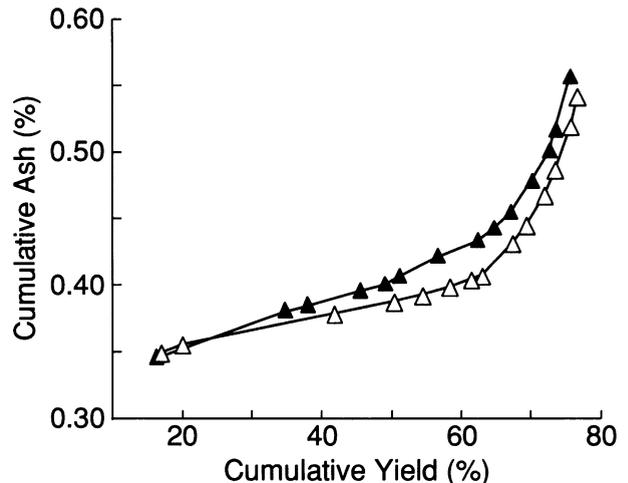
Fig. 2. Cumulative ash curves that illustrate the maximum range of mill performance among replicate millings of a No. 1 Canada western red spring wheat achieved by manipulating mill settings. The flatter curve ( $\Delta$ ) is indicative of better milling performance than the steeper curve ( $\blacktriangle$ ). Ash content expressed on 14% moisture basis; flour yield expressed as proportion of clean wheat on constant moisture basis.
