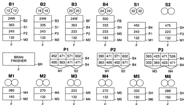
Fig. 1. Grain Research Laboratory pilot mill hard wheat flow. Nitex sieve apertures given in microns. 24 wire (W) aperture 730 microns. Roll fluting expressed as corrugations per inch. B = break, S = sizing, M = middling, P = purifier, F = flour, BF = bran finisher, SH = shorts, BR = bran, FB = fine bran.
