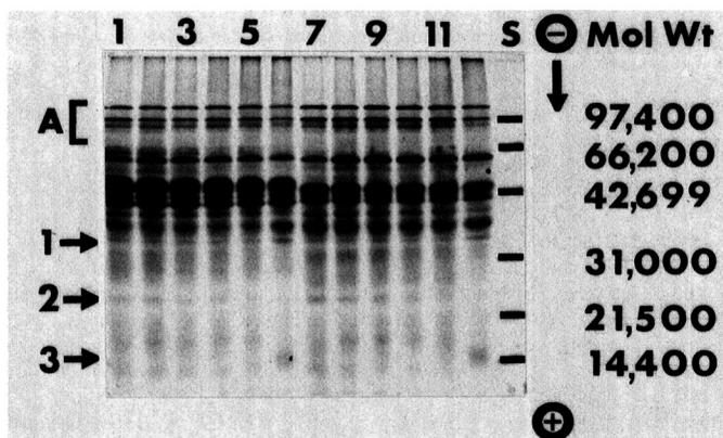
Fig. 7. Sodium dodecyl sulfate-polyacrylamide gel electrophoresis patterns of residue of Vic (patterns 1–6) and Rugby (patterns 7–12) samples: S, molecular weight standards; 1 and 7, semolina; 2 and 8, 40°C-dried spaghetti; 3 and 9, 60°C-dried spaghetti; 4 and 10, 70°C-dried spaghetti; 5 and 11, 80°C-dried spaghetti; 6 and 12, 90°C-dried spaghetti. A and arrows 1–3 = regions showing differing effects of increased drying temperature.
