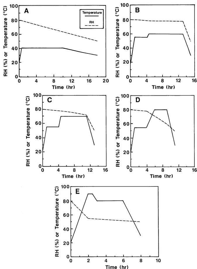
Fig. 1. Drying curves of spaghetti processed from Vic and Rugby semolina. A-E, Spaghetti dried at 40, 60, 70, 80, and 90°C, respectively.
