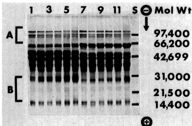
Fig. 6. Sodium dodecyl sulfate-polyacrylamide gel electrophoresis patterns of glutenin of Vic (patterns 1–6) and Rugby (patterns 7–12) samples: S, molecular weight standards; 1 and 7, semolina; 2 and 8, 40°C-dried spaghetti; 3 and 9, 60°C-dried spaghetti; 4 and 10, 70°C-dried spaghetti; 5 and 11, 80°C-dried spaghetti; 6 and 12, 90°C-dried spaghetti. A and B = regions showing differing effects of increased drying temperature.
