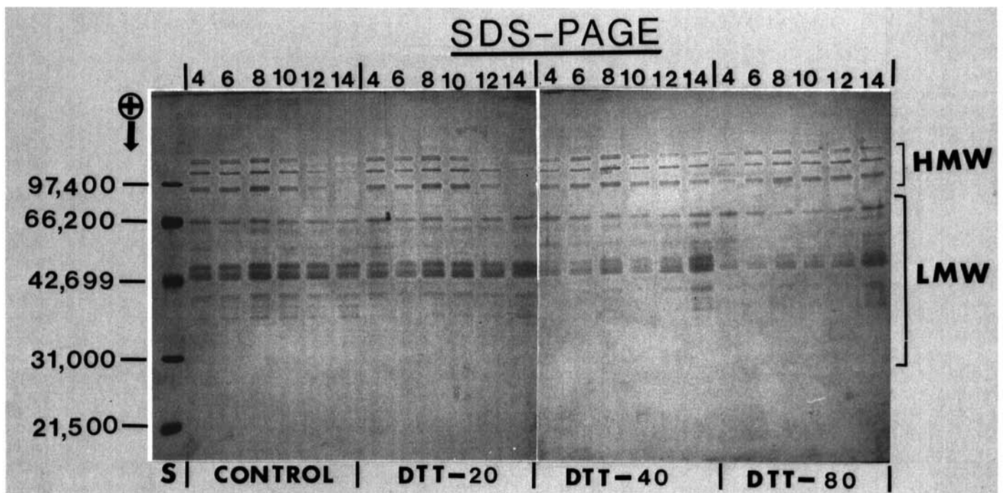
Fig. 2. Sodium dodecyl sulfate-polyacrylamide gel electrophoresis patterns of reduced (5% excess reducing agent) proteins eluted from the origins of the stacking gels and the resolving gel of Figure 1, patterns 1–4. The numbers 4–14 (top) indicate the origin of the gel concentration (Fig. 1) from which the pattern was obtained. The dough treatments used (bottom) are: control (with N -ethylmaleimide) and 20, 40, and 80 \mu\text{mol} of dithiothreitol (DTT). S = molecular weight standards. LMW = low molecular weight subunits. HMW = high molecular weight subunits.
