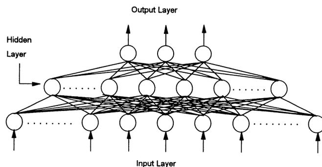
Fig. 1. Architecture of a feedforward backpropagation neural network.
