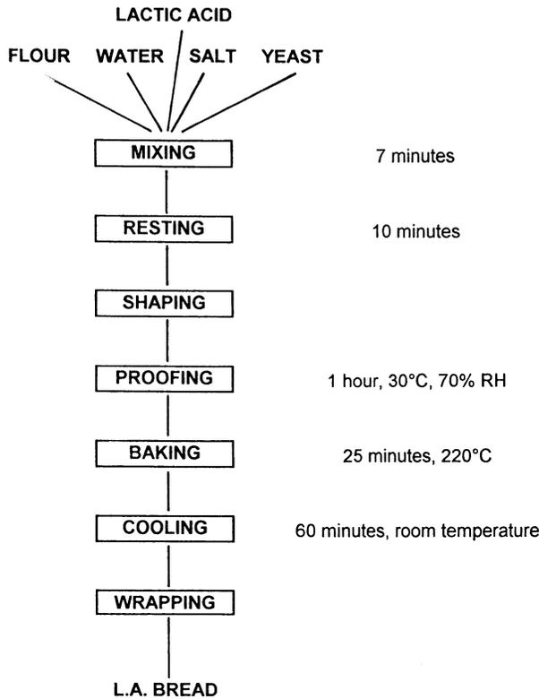
Fig. 3. Flow diagram for preparation of straight-dough bread acidified with lactic acid (LA).
