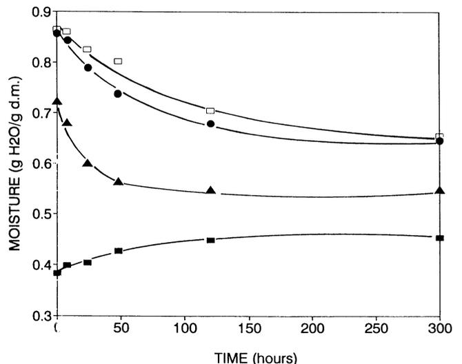
Fig. 6. Effect of time on the moisture of lactic acid type bread in the various region of the central slice. ■ = crust; ▲ = near-crust; ● = middle; □ = center.
