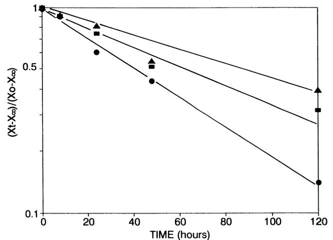
Fig. 8. Bread drying curves plotted according to Equation 1. ■ = yeast bread; ▲ = sour-dough bread; ● = lactic acid bread.
