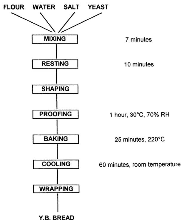
Fig. 1. Flow diagram for preparation of straight-dough bread (YB).
