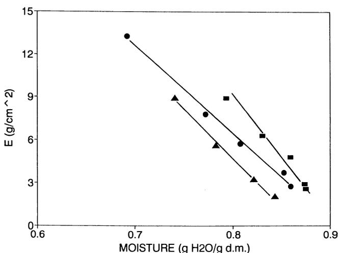
Fig. 11. Modulus of elasticity vs. bread moisture content. ■ = yeast bread; ▲ = sour-dough bread; ● = lactic acid bread.
