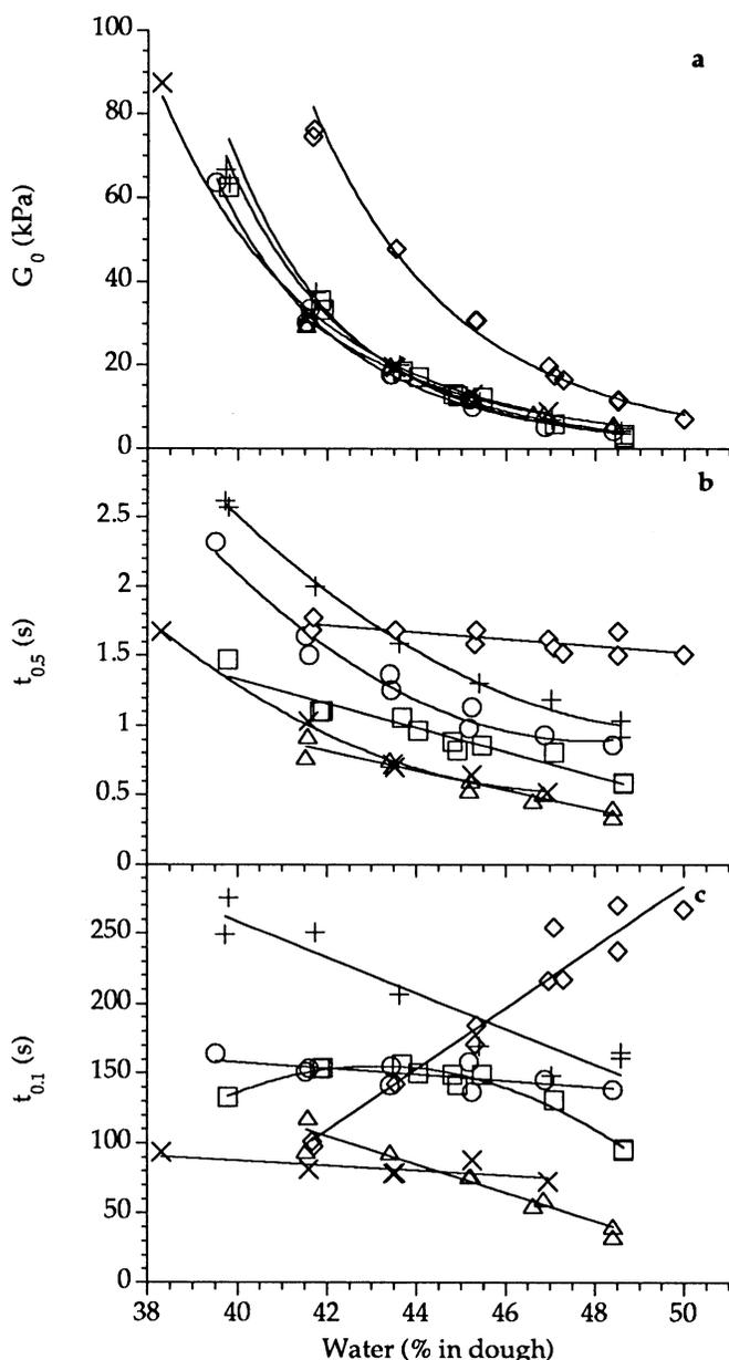
Fig. 5. Influence of dough water content on a, stress-relaxation modulus ( $G_0$ ); b and c, stress-relaxation times ( $t_{0.5}$  and  $t_{0.1}$ , respectively). Symbols as in Fig. 3.
