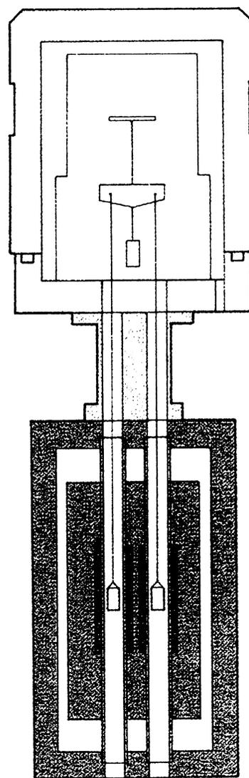
Fig. 1. Schematic view of thermogravimetry apparatus (Setaram TG-DSC 111) used for determination of water losses.
