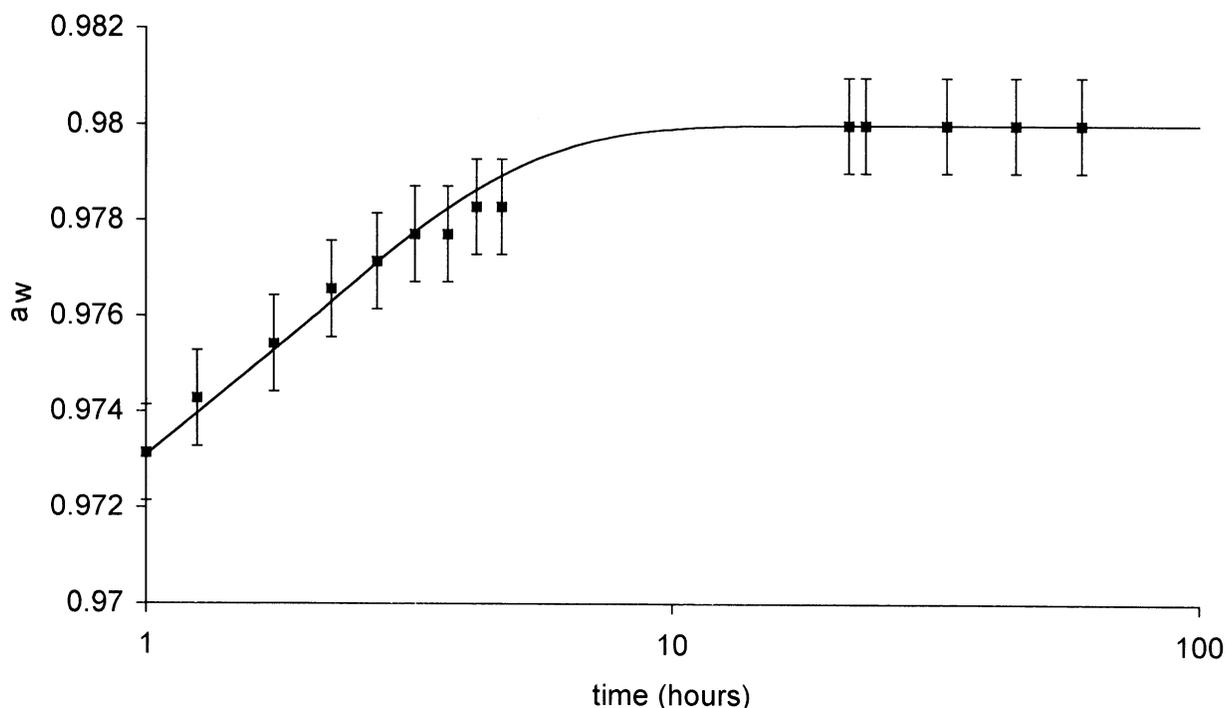
Fig. 9. Trend of the water activity ( $a_w$ ) vs. aging for control bread samples.
