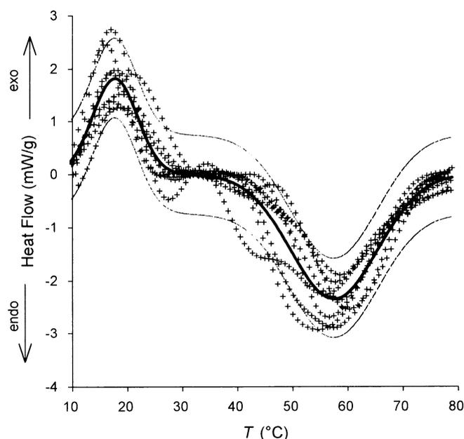
Fig. 2. Average of differential scanning calorimetry traces (2°C/min heating rate) from eight control bread samples stored at 20°C for 5 hr. --- = Relevant 95% prediction limits. — = Relevant average fit.
