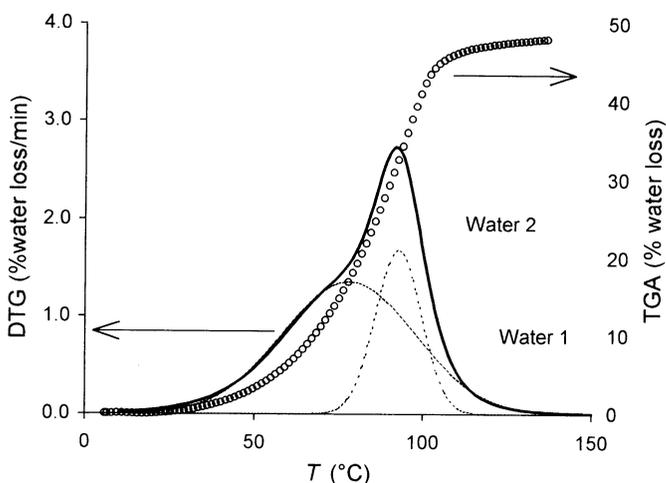
Fig. 5. Thermogravimetry (TGA) and derivative TG (DTG) traces recorded with 2°C/min scanning rate on 5-hr aged control bread samples. Dotted and dashed lines represent deconvoluted components of the DTG curve.
