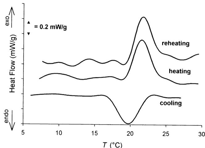
Fig. 6. Differential scanning calorimetry traces of a control bread sample (2°C/min heating or cooling rate) in a three-run cycle over a 5–30°C temperature range.
