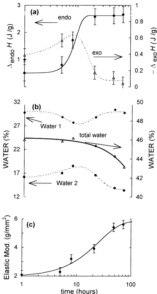
**Fig. 7.** Control bread crumb changes observed in the course of aging. **a**, Endo- and exothermic effect; **b**, water-1, water-2, and total water reported from thermogravimetry data; **c**, elastic modulus.
