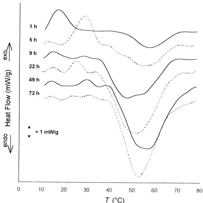
**Fig. 3.** Differential scanning calorimetry traces of control bread samples ( $2^{\circ}\text{C}/\text{min}$  heating rate) at different storage times. Traces are shifted to one another for the sake of clarity.
