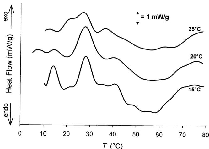
**Fig. 4.** Differential scanning calorimetry traces of control bread samples ( $2^{\circ}\text{C}/\text{min}$  heating rate) stored for  $8$  hr at different temperatures. Traces are shifted to one another for the sake of clarity.
