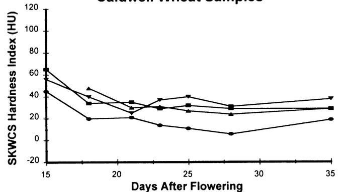
Fig. 4. Hardness index vs. stage of development for Caldwell wheat. Air-dried (■), oven-dried (▼), lyophilized (●), and freeze-thawed (▲).
