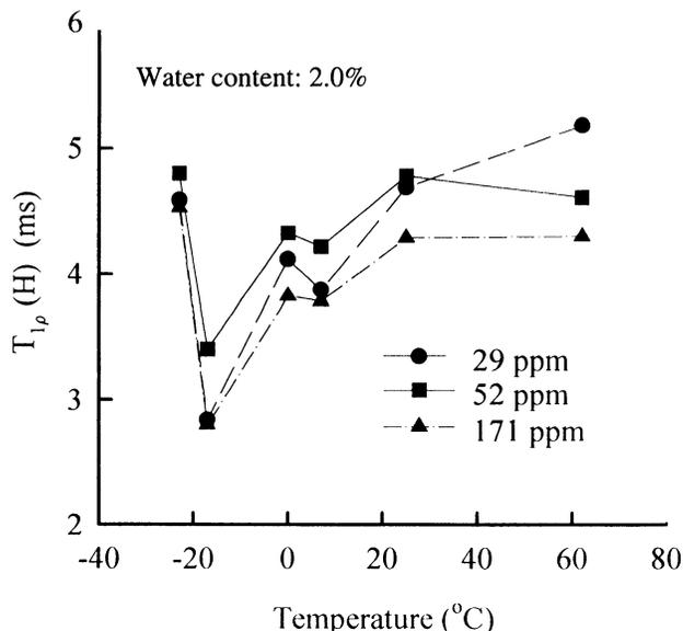
Fig. 7. Proton rotating frame relaxation times [ $T_{1\rho}(H)$ ] of heated wheat gluten at 2.0% water content as a function of temperature. Lines are for presentation clarity.
