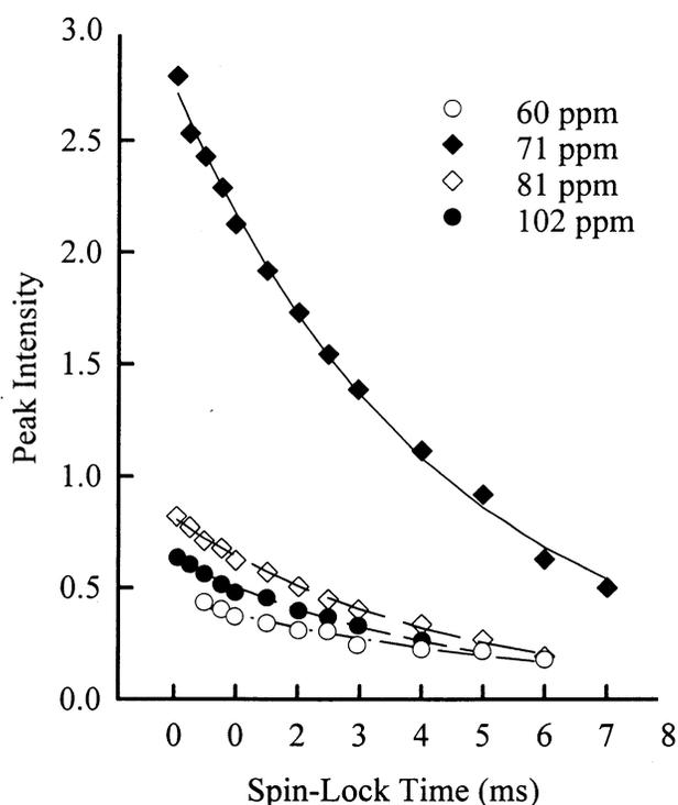
Fig. 4.  $^{13}\text{C}$  nuclear magnetic resonance intensities for heated waxy starch at 12.5% water content as a function of spin-lock time at ambient temperature. Lines are the best fits from the one-component model.
