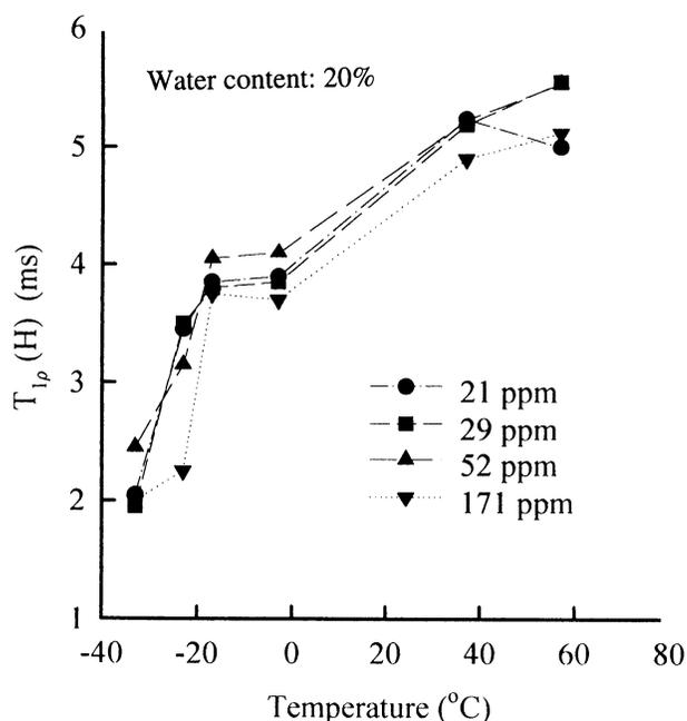
Fig. 8. Proton rotating frame relaxation times [ $T_{1\rho}(H)$ ] for heated wheat gluten at 20.0% water content (MC) as a function of temperature. Lines are for presentation clarity.
