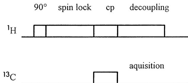
Fig. 1. Pulse sequences used for the measurement of proton rotating frame relaxation times [ $T_{1\rho}(\text{H})$ ]. Proton magnetization was spin-locked in the rotating frame for various times, and the decay of magnetization was measured using  $^{13}\text{C}$  cross-polarization (cp).  $^{13}\text{C}$  spectra were obtained with zero spin-locked time.
