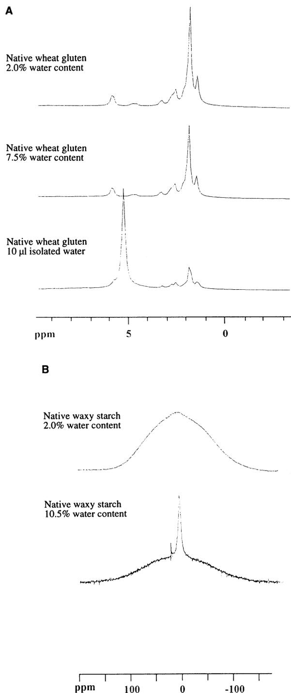
**Fig. 6.** Wideline  $^1\text{H}$  nuclear magnetic resonance of native wheat gluten (A) and native waxy starch (B) at ambient temperature.
