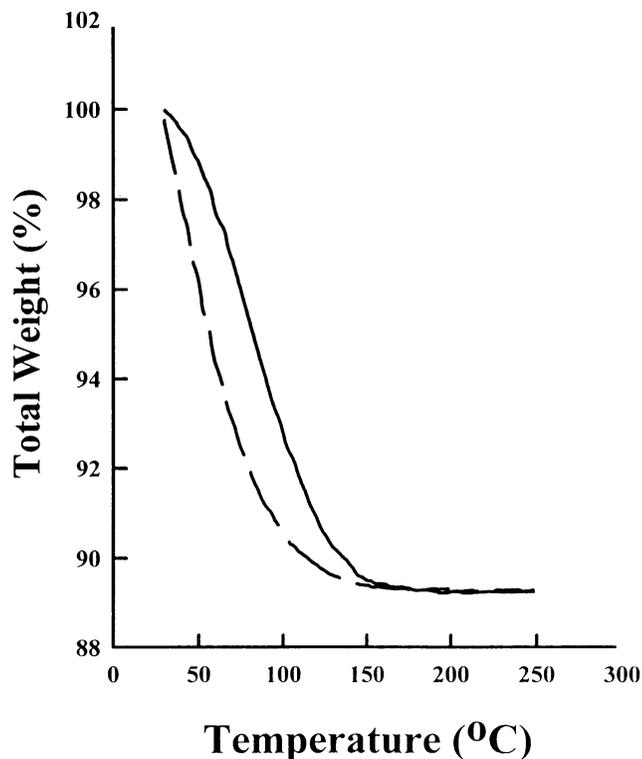
Fig. 2. Thermogravimetric analysis curves for moisture content in native waxy corn starch heated at  $2^\circ\text{C}/\text{min}$  (---) and at  $20^\circ\text{C}/\text{min}$  (—). Moisture content was measured by the weight loss at  $180^\circ\text{C}$ .
