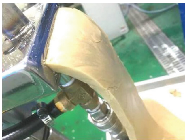
Fig. 3. A high-moisture meat analogue sample exiting a cooling die.
