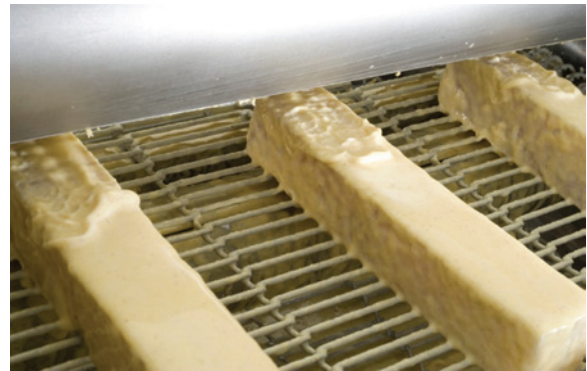
Fig. 4. Application of batter on fish sticks. (Photo courtesy of GEA Food Solutions)
