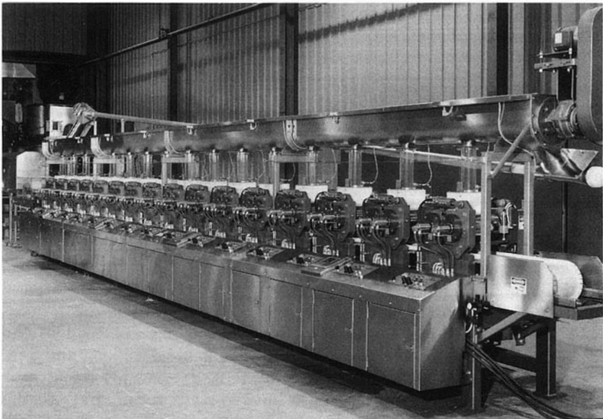
Figure 6. Sixteen-station shredded wheat cereal biscuit forming line. This state-of-the-art line can produce 2,500 lb (1,135 kg) of dry, uncoated shredded wheat mini-biscuits per hour. (Courtesy Wolverine Proctor and Schwartz)
