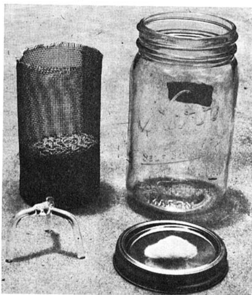
Fig. 1. Storage container for maintaining rice at a high relative humidity.
