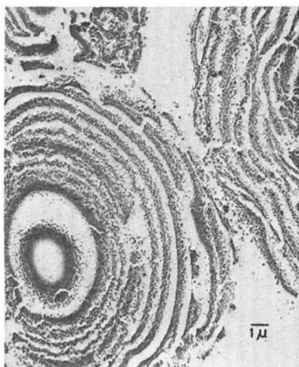
Fig. 4 (upper left). Unmodified amylo maize starch; montage of three electron micrographs; as-is.
