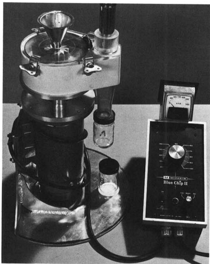
Fig. 2. Laboratory decortivating mill with drive and speed controller.
