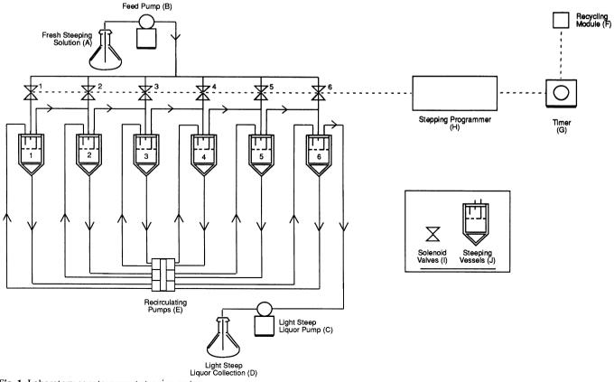
by a timer and a recycle module. The solution was advanced to succeeding steeping vessels by an electromechanical multicircuit stepping programmer.
