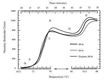
Fig. 2. Brabender viscoAmylograph curves of laboratory-isolated starches from continuous countercurrent steeping with and without multiple enzymes, showing peak pasting temperature (A), peak viscosity (B), peak viscosity at  $95^{\circ}$ C (C), extent of breakdown (D), amount of setback (E), and gelatinization onset temperature (To).
