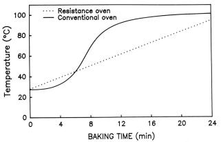
Fig. 1. Temperature profile during baking in an electric resistance oven.
