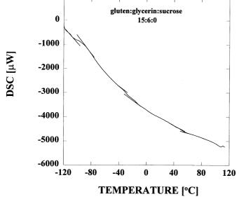
Fig. 1. Differential scanning calorimetry (DSC) thermogram of wheat gluten-glycerin-sucrose film at a ratio of 15:6:0 (w/w) showing a series of decreases in the baseline upon heating and indicating a change in heat capacity.
