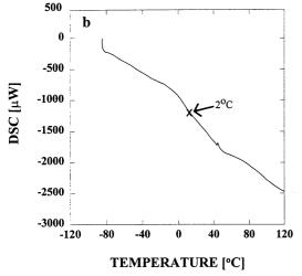
Fig. 3. Thermograms for wheat gluten-glycerin-sucrose film at a ratio of 15:0:6 (w/w), conditioned at 50% rh and 25°C, moisture content 9.3% (wb). Dynamic mechanical analysis (a) records storage modulus (E'), loss modulus (E''), and loss angle (tan  $\delta$ ) plotted against temperature. Differential scanning calorimetry (b) shows no ice melting peak.
