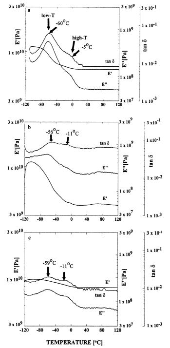
Fig. 2. Dynamic mechanical analysis thermograms for wheat glutenglycerin-sucrose films at various ratios (w/w) and moisture contents (%, wb). a, 15:6:0 (18.7%). b, 15:4:2 (14.4%). c, 15:3:3 (9.6%) conditioned at 50% rh and 25°C for two days. Storage modulus (E'), loss modulus (E''), and loss angle (tan  $\delta$ ) were recorded and plotted against temperature.
