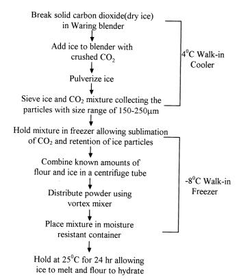
Fig. 1. Flow diagram of the powder method of making undeveloped dough.
