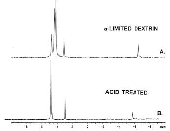
Fig. 8. <sup>31</sup>P nuclear magnetic resonance spectra of  $\alpha$ -limited dextrin prepared from potato starch: A, without acid hydrolysis. Signals between 3.5 and 5.0 ppm are phosphate monoesters. B, with acid hydrolysis. Signal at 4.9 ppm is glucose-6-phosphate. Signal at 3.0 ppm is inorganic phosphate.
