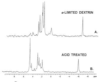
**Fig. 10.** <sup>31</sup>P nuclear magnetic resonance spectra of normal rice starch  $\alpha$ limited dextrin: **A**, without acid hydrolysis. Signals between -1.0 and 1.0 ppm are phospholipids. **B**, with acid hydrolysis. Signal at 4.6 ppm is glycerophosphate. Signals between 1.0 and 3.0 ppm are phosphoproteins.
