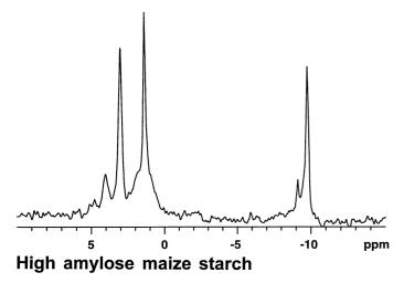
**Fig. 6.** <sup>31</sup>P nuclear magnetic resonance spectrum of  $\alpha$ -limited dextrin prepared from high-amylose maize starch (50% amylose). Signal at 9.8 ppm is an internal reference standard (nicotinamide adenine dinucleotide, 12.5 mg).
