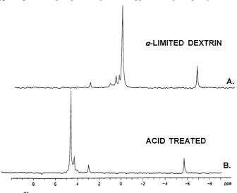
Fig. 9. <sup>31</sup>P nuclear magnetic resonance spectra of  $\alpha$ -limited dextrin prepared from wheat starch: A, without acid hydrolysis. Signals between -1.0 and 1.0 ppm are phospholipids. B, with acid hydrolysis. Signal at 4.6 ppm is glycerophosphate. Signal at 3.0 ppm is inorganic phosphate.
