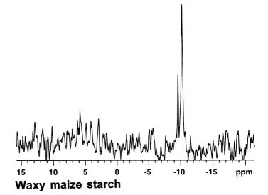
Fig. 7. <sup>31</sup>P nuclear magnetic resonance spectrum of  $\alpha$ -limited dextrin prepared from waxy maize starch. Signal at 10.2 ppm is an internal reference standard (nicotinamide adenine dinucleotide, 0.3125 mg).
