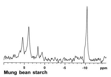
Fig. 3. <sup>31</sup>P nuclear magnetic resonance spectrum of  $\alpha$ -limited dextrin prepared from mung bean starch. Signal at 10.2 ppm is an internal reference standard (nicotinamide adenine dinucleotide, 1.25 mg).
