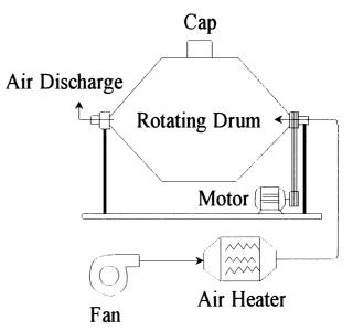
Fig. 1. Side-view drawing of Miag Laboratory wheat conditioner. The air-flow meter and temperature controller and recorder are not shown.
